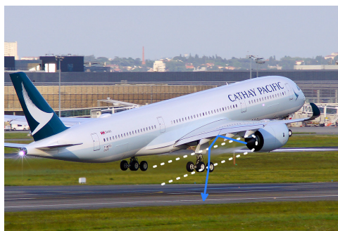
Figure 1.1: Airbus A350-900 XWB [5] at take-off producing a jet of exhaust gas traversed by an acoustic wave (blue arrow) from the engine, reflected on the wing and crossing the jet flow.
