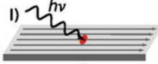
Figure 11 : Adapted from [70], a representation of the photon absorption process in a thin superconducting wire. The breaking of Cooper pairs occurs when a photon of energy h\nu is absorbed, resulting in a normal-conducting hotspot. The arrows denote a constant bias current I_b .
