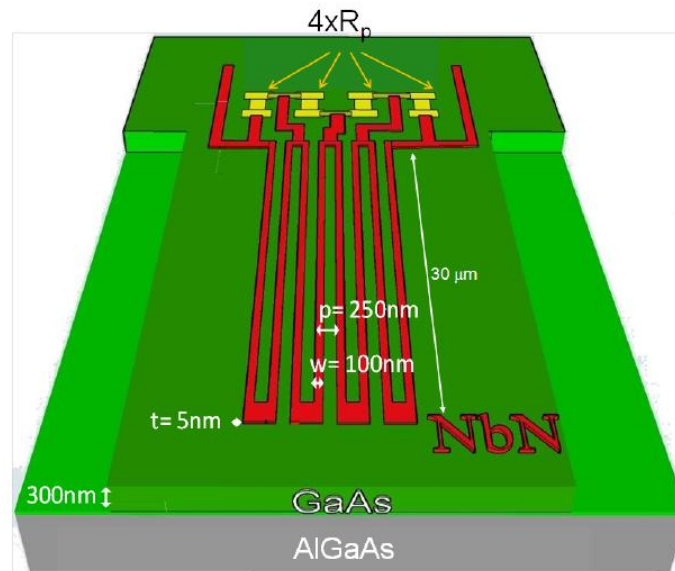
Figure 42: Schematic of a waveguide photon-number-resolving detector consisting of four nanowires in parallel
