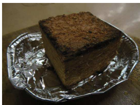
Figure 4-16. S6 sample after ignition time test
