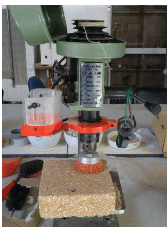
Figure 4-2. Dry abrasion test
