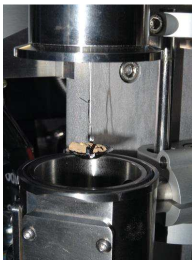
Figure 3-20. Sample holder in its opened cell (here CC3 sample)
