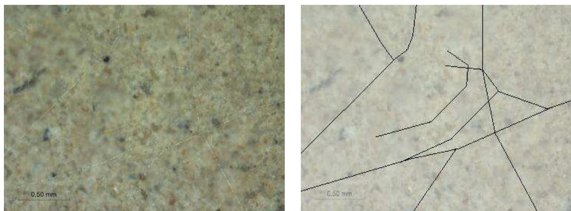
Figure 4-23. Hyphae of a FWAS sample at 93% RH and 30°C after 12 weeks: microscopic photo (left) and manual identification of hyphae routes (right)
