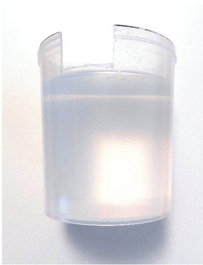
Figure 6-18: Picture of silicon phantom
