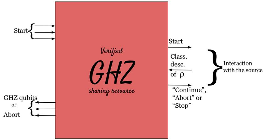
Figure 3.16: Verified  $\epsilon$ -GHZ sharing resource for 3 parties. It takes start signals as input from the parties on the left interface then interacts with the source on the right interface. It outputs either a shared quantum state  $\epsilon$ -close to the GHZ state or an abort signal to the parties.
