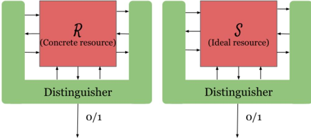
Figure 3.3: A distinguisher interacting with  $\mathcal{R}$  and  $\mathcal{S}$ . It has access to a complete description of the two systems and can choose the inputs of all players, receive their outputs and simultaneously fulfill the role of an adversary. After interaction, it must guess which resource is which. Replacing  $\mathcal{R}$  by Fig. 3.1 and  $\mathcal{S}$  by Fig. 3.2, no distinguisher is able to guess between the two resources.
