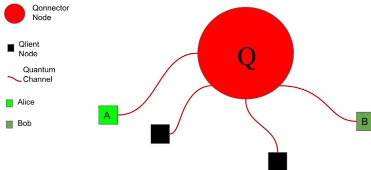
Figure 5.1: The Quantum City topology. It is a photonic star quantum network with a special node in the middle, the Qconnector, that has advanced quantum capabilities. Each end node (Qlient) has very limited quantum capabilities and is connected to the Qconnector through an optical fiber. The Quantum City allows for Qlients to perform quantum protocols via the Qconnector.
