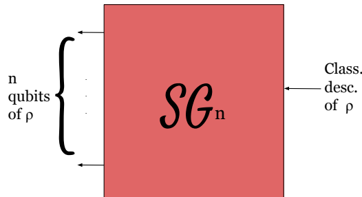
Figure 3.8: State generator resource.
