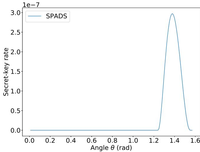
Figure 4.11: (Color on-line) Secret-key rate as a function of the  $\theta$  angle for the SPADS scheme for the total distance of  $12.5L_0$ , where  $L_0 = 0.542$  km. We see that due to more noisy processes the range of  $\theta$  that allows us to generate key is much more restricted than for the single-photon scheme. For each value of  $\theta$  the secret-key rate is optimized over the cutoff  $n^*$  and the time-window  $t_w$ .
