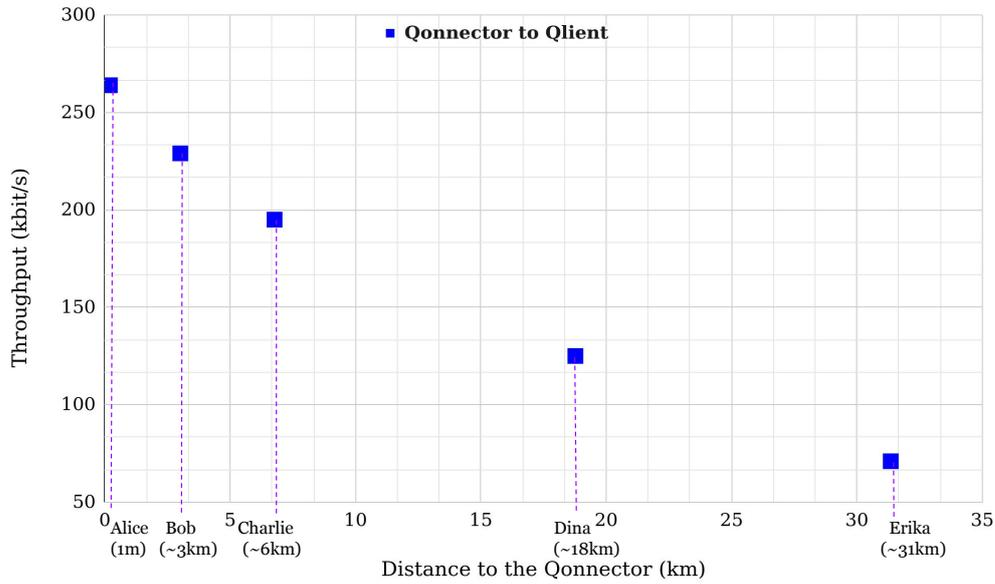
Figure 5.5: Throughput of BB84 state transmission from the Qconnector to the Qlients (blue squares). The throughput is the number of sifted key bits per second shared between each Qlient and the Qconnector.
