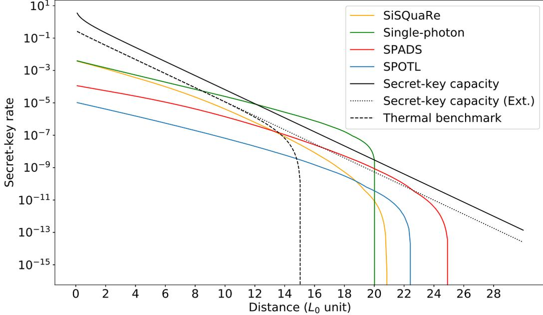
Figure 4.15: (Color on-line) Rate of all studied quantum repeater schemes as a function of the distance between Alice and Bob, expressed in the units of  $L_0 = 0.542$  km. We also plot the different benchmarks from Section 4.5. We see that the single-photon scheme outperforms the secret-key capacity. For the achievable rates the secret-key rate is optimized over the cutoff  $n^*$ , the angle  $\theta$  and the time-window  $t_w$  independently for each distance.
