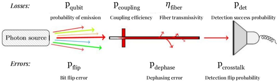
Figure 5.2: Photon loss and error model for the emission, sending and measurement of a qubit.
