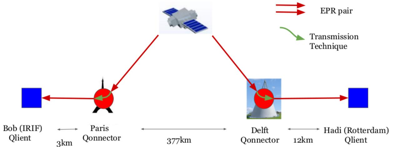
Figure 6.11: QKD between Bob and Hadi: Untrusted nodes. Here the satellite performs the BBM92 protocol directly with the Qlients. The Qconnectors are used as transmitting stations, that couple the photons arriving from the satellite into a fiber and send them to the QClients.
