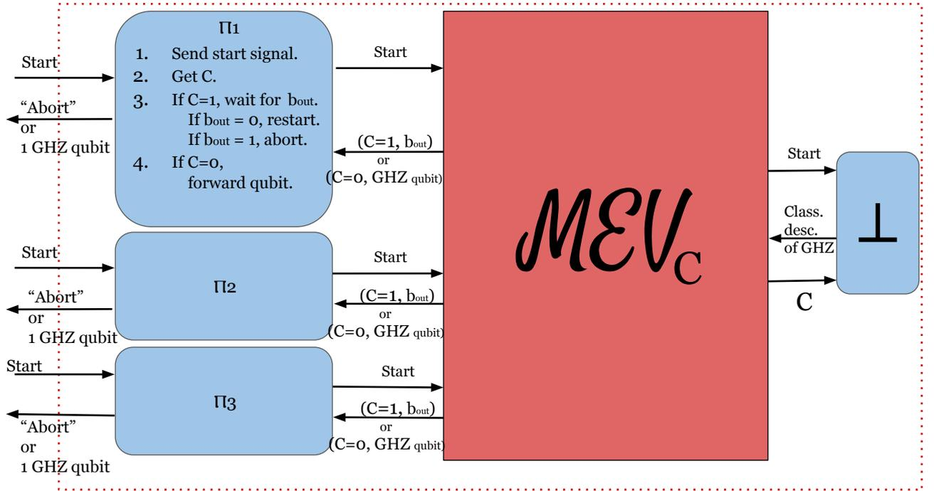
Figure 3.15: Multi-round verification resource  $\Pi_{[n]}\mathcal{MEV}_C \perp$  for 3 parties (in the red dotted square). It takes start signals as input and outputs either a shared quantum state  $\epsilon$ -close to the GHZ state or an abort signal.
