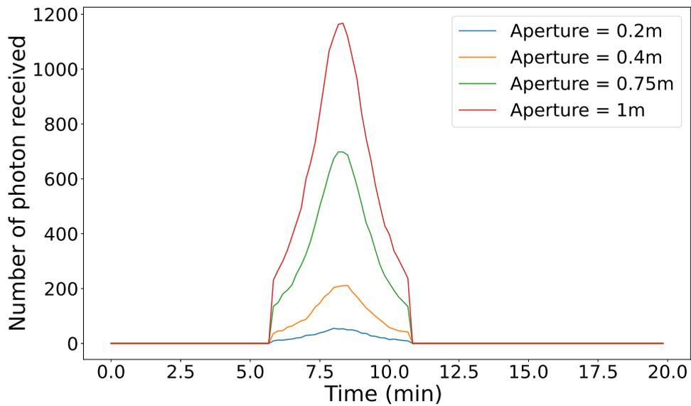
Figure 6.8: Effect of the aperture radius of the receiving telescope  $R_x$  on the number of photonic qubits arriving from the Micius satellite.
