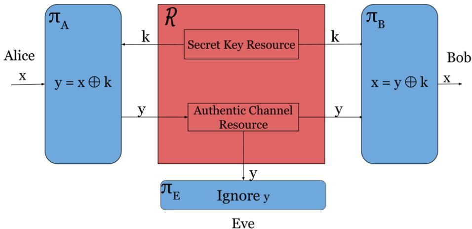
Figure 3.1: Concrete One Time Pad resource  $\pi_A \pi_B \mathcal{R} \pi_E$ : Alice has access to the left interface, Bob to the right interface and Eve to the down interface.  $\mathcal{R}$  is the resource composed of a secret key resource and an authentic channel resource in parallel. Protocols are represented in blue,  $\pi_E$  being the protocol of an honest Eve that blocks the input  $y$  from the authenticated channel resource.
