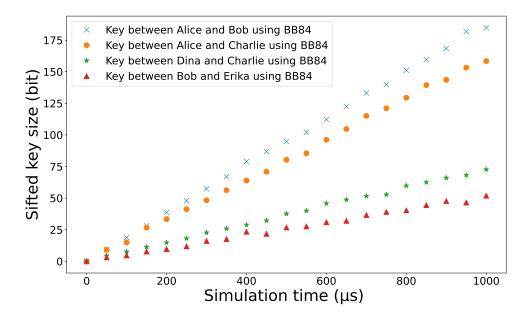
Figure 5.7: Comparison between the number of successful BB84 qubit transmission from some Qlients to others through the Qonnector.
