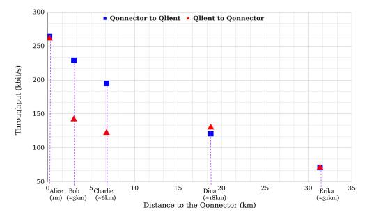
Figure 5.9: Throughput of BB84 state transmission from the Qonnector to the Qlients (blue squares) and from the Qlients to the Qonnector (red triangles) with the modified set of parameter. The throughput represent the number of sifted key bits per second shared between each Qlient and the Qonnector.
