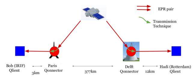
Figure 6.11: QKD between Bob and Hadi: Untrusted nodes. Here the satellite performs the BBM92 protocol directly with the Qlients. The Qonnectors are used as transmitting stations, that couple the photons arriving from the satellite into a fiber and send them to the Qlients.
