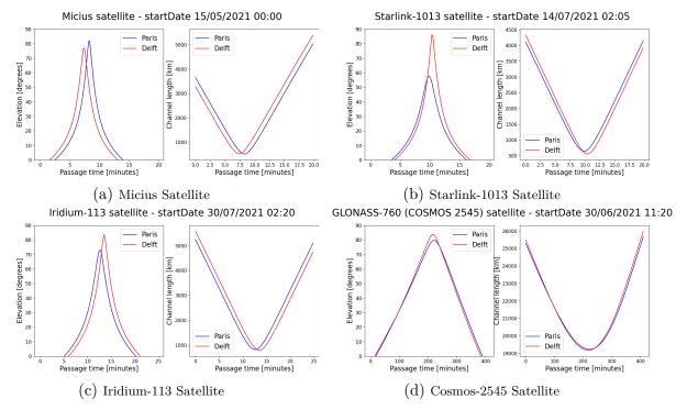
Figure 6.3: Elevation and distance to Paris and Delft of the Micius, Starlink, Iridium and Cosmo satellites in the time frame considered.
