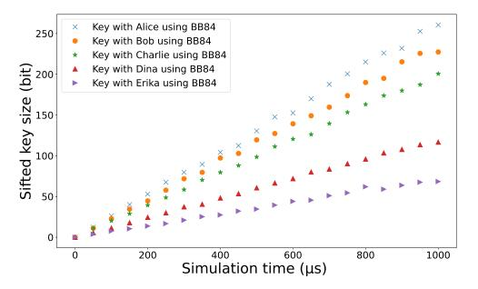
Figure 5.6: Comparison between the number of successful BB84 qubit transmission from the Qonnector to every Qlient of our network.
