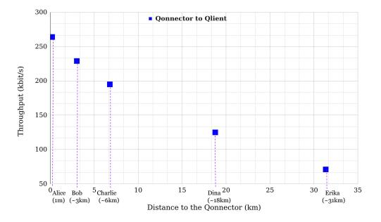
Figure 5.5: Throughput of BB84 state transmission from the Qonnector to the Qlients (blue squares). The throughput is the number of sifted key bits per second shared between each Qlient and the Qonnector.
