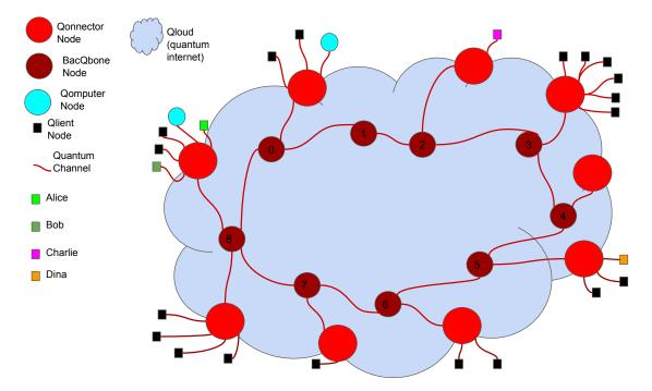
Figure 6.1: Schematic of a Qloud: Quantum cities connected through a backbone network of satellites (BacQbone nodes). A Quantum City is formed by a powerful central node (Qonnector nodes) used as a server allowing end users (Qlients) to enjoy quantum-enhanced functionalities. The end users can also be powerful quantum machines (Qomputer nodes).
