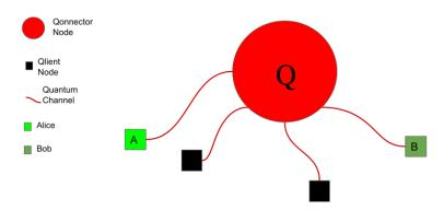
Figure 5.1: The Quantum City topology. It is a photonic star quantum network with a special node in the middle, the Qonnector, that has advanced quantum capabilities. Each end node (Qlient) has very limited quantum capabilities and is connected to the Qonnector through an optical fiber. The Quantum City allows for Qlients to perform quantum protocols via the Qonnector.
