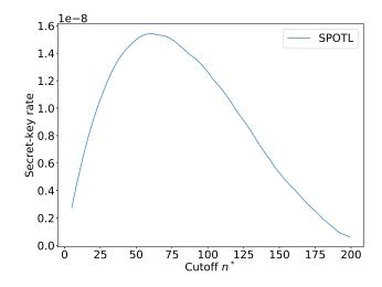
Figure 4.14: (Color on-line) Secret-key rate as a function of the cut-off for the SPOTL scheme for the total distance of  $12.5L_0$ , where  $L_0 = 0.542$  km. We see that due to the large number of noisy operations, this scheme requires a low cut-off in order to be able to generate key. For each value of the cutoff  $n^*$  we optimize the secret-key rate over the time-window  $t_w$  and the  $\theta$  angle.
