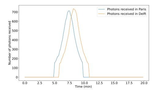
Figure 6.10: Average number of photons received in Paris and Delft for approximately 3000 photons sent from the satellite at each orbit point.
