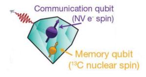
Figure 1.2: Schematic of an NV center in a diamond. It contains two addressable qubits: the spin of an electron with an optical interface coupled to a <sup>13</sup>C memory qubit.
