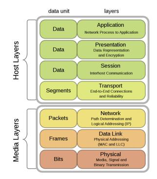
Figure 1.3: The 7 layers of the OSI model that partition the flow of data
