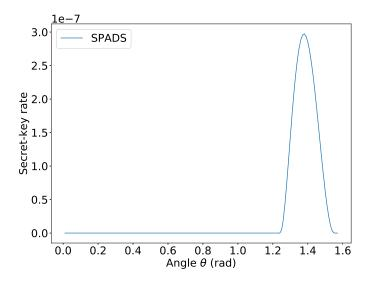
Figure 4.11: (Color on-line) Secret-key rate as a function of the  $\theta$  angle for the SPADS scheme for the total distance of  $12.5L_0$ , where  $L_0 = 0.542$  km. We see that due to more noisy processes the range of  $\theta$  that allows us to generate key is much more restricted than for the single-photon scheme. For each value of  $\theta$  the secret-key rate is optimized over the cutoff  $n^*$  and the time-window  $t_w$ .
