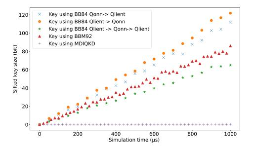
Figure 5.11: Comparison between different QKD protocols between Charlie and Dina. We show the size of the sifted key between the two Qlient using different QKD protocol as a function of the simulation time.
