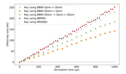
Figure 5.10: Comparison between different QKD protocols between Alice and Bob. We show the size of the sifted key between the two Qlient using different QKD protocol as a function of the simulation time.
