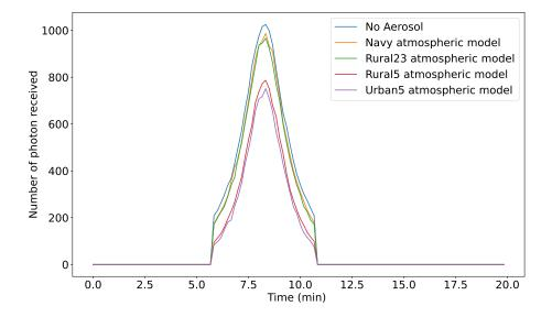
Figure 6.5: Effect of different aerosol models on the number of photonic qubits arriving from the Micius satellite.
