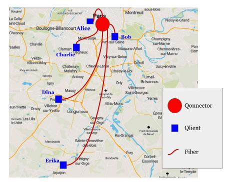
Figure 5.3: Paris Quantum City: Five Qlients are connected through optical fibers to a Qonnector located at Sorbonne Université (SU) campus. The length of the fiber are 1m for the link Alice-Qonnector, 3km for the link Bob-Qonnector, 7km for the link Charlie-Qonnector, 19km for the link Dina-Qonnector and 32km for the link Erika-Qonnector.
