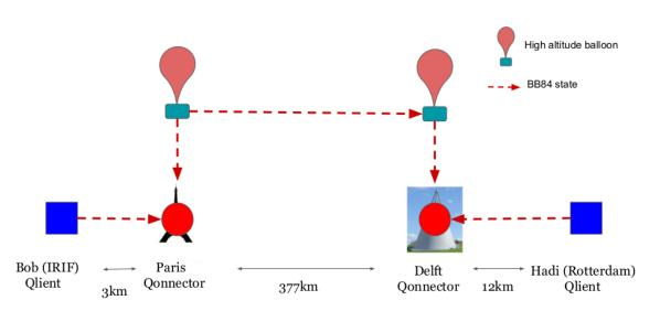
Figure 6.13: A trusted node QKD scenario between two Qlients using two high-altitude balloons over the Qonnectors. We suppose that the drones are 10km above each Qonnector.
