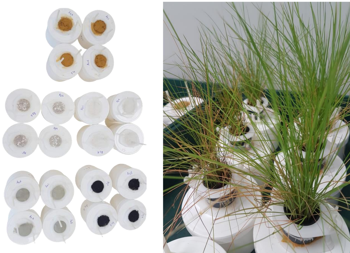
Figure 8 : RHIZOtest device experiment setting
