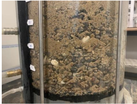
Figure 4.27 Couche aval de la configuration aval
