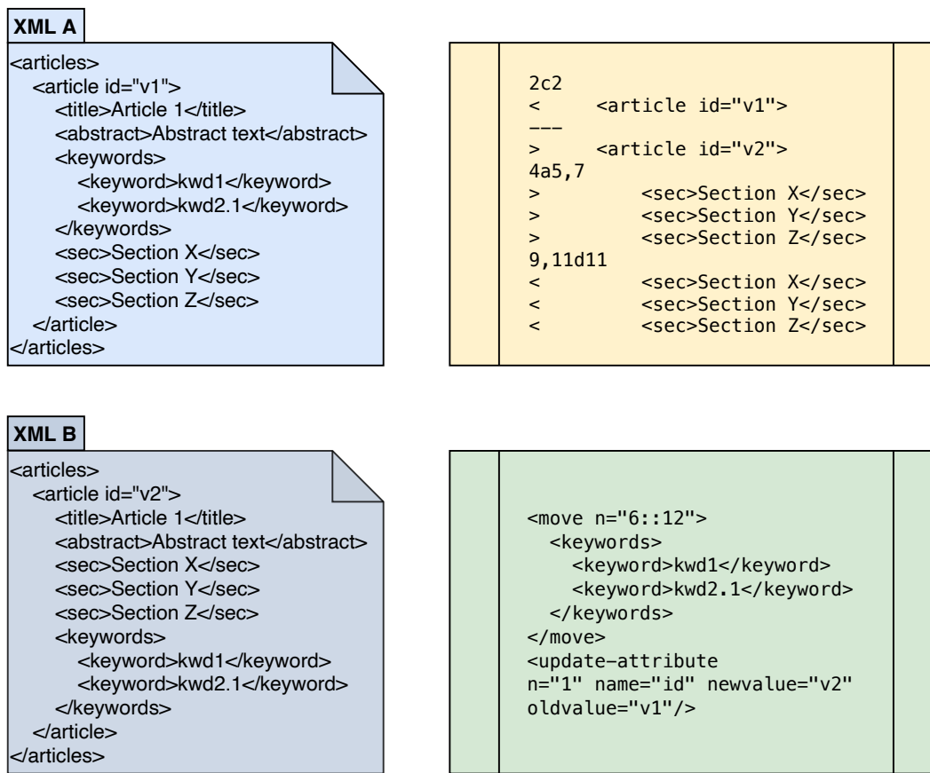
Figure 2-1: line-based text diff (top-right) VS XML diff (bottom-right) XML compare.
