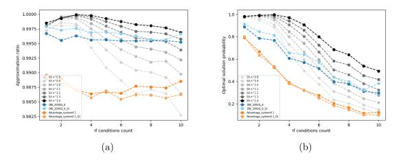
Figure 7.3: Benchmark of the QUBO resolution by D-Wave systems and SA for IF chains from 1 to 10 IF conditions. Each D-Wave simulation is done with and without GI (Gauge Inversion). n is the number of blocks in the if chain. SA number of iteration per temperature step is expressed according to n. a) Mean of approximation ratio. b) Mean of the probability to get the optimal solution.
