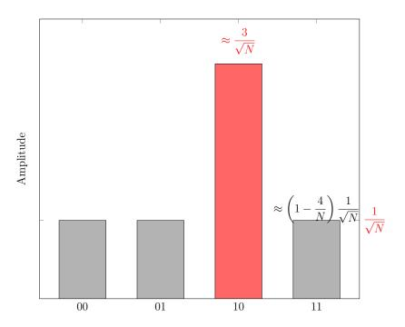
Figure 2.8: Amplification of the probability amplitude of the target element.
