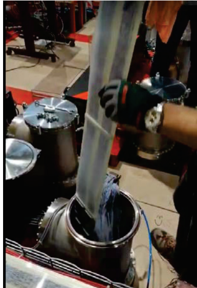
FIGURE 4.6: Access to a front-end cryogenic amplifier card in a signal feed-through chimney
