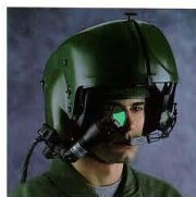
Figure 1. Integrated Helmet and Display Sighting System (IHADSS) used by United States Army Apache AH-64 pilots
