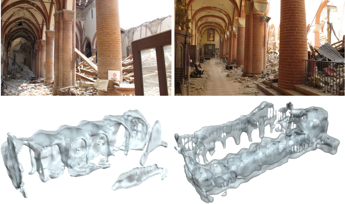
Figure 4.4: Snapshots of the two destroyed historical sites in which the robot navigated and corresponding 3D maps.
