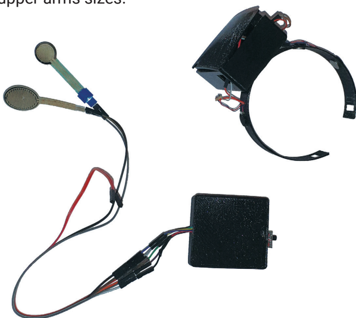
Figure 7.8. Third and latest iteration of the sensory feedback system. The two parts are communicating using two Bluno Beetle boards from DFRobot.
