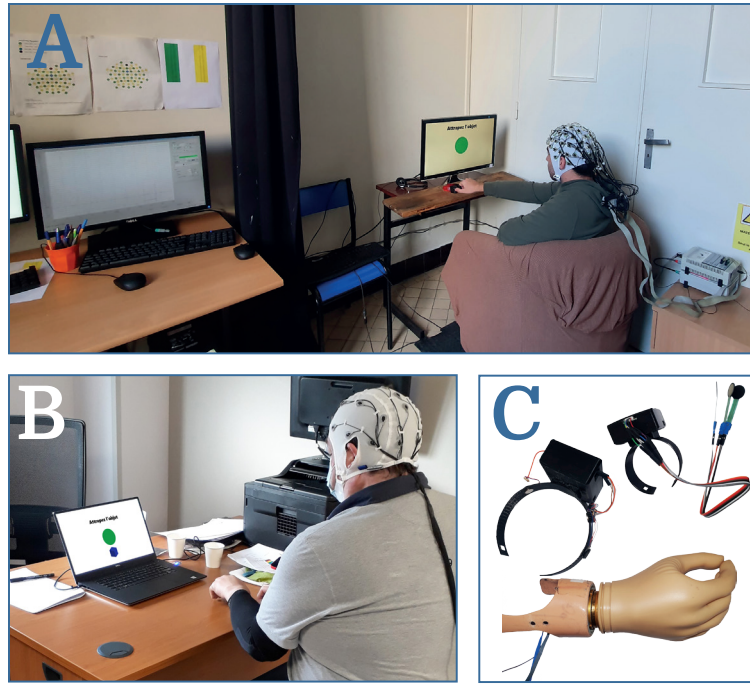
Figure 4.1. Experimental setups used during the experiments. A. Experimental setup with able-bodied subjects at Université Paris Cité. B. Experimental setup with amputee subjects at IRMA. C. Prosthesis and sensory feedback devices used during the second and third session with the amputees.
