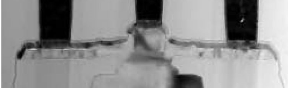
Figure I.9 | TEM cross section of the Elevated Extrinsic Base - Selective Epitaxial growth (EBL-SEG) HBT presented by Manger et al. [40].
