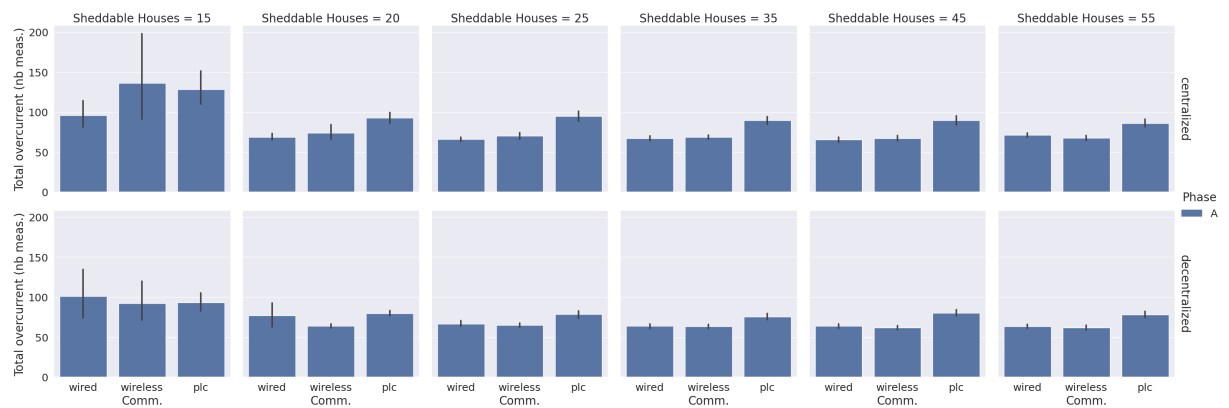
Figure 5.2: Total overcurrent versus number of sheddable houses. The current threshold is set to 0.5 kA, message size to 1 kB, shedding duration to 60 s, sampling period to 20 s and latency to 10 ms.
