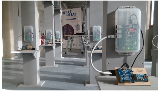
Figure 6.13: Physical IoT devices in the Saclay site of the FIT IoT-LAB. Source: [4].
