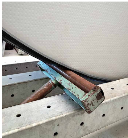
Figure 7.12: Roller used to hold the panel vertically. The linking forces applied to the panel are in-plane.
