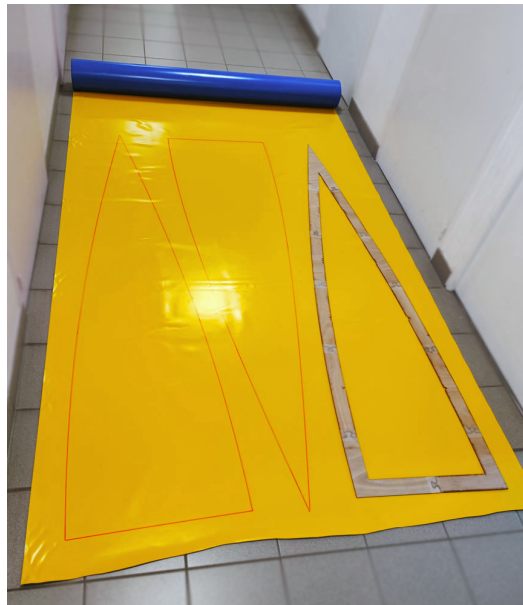
Figure 7.6: Marking of the outline of each meridian section using the wooden template.
