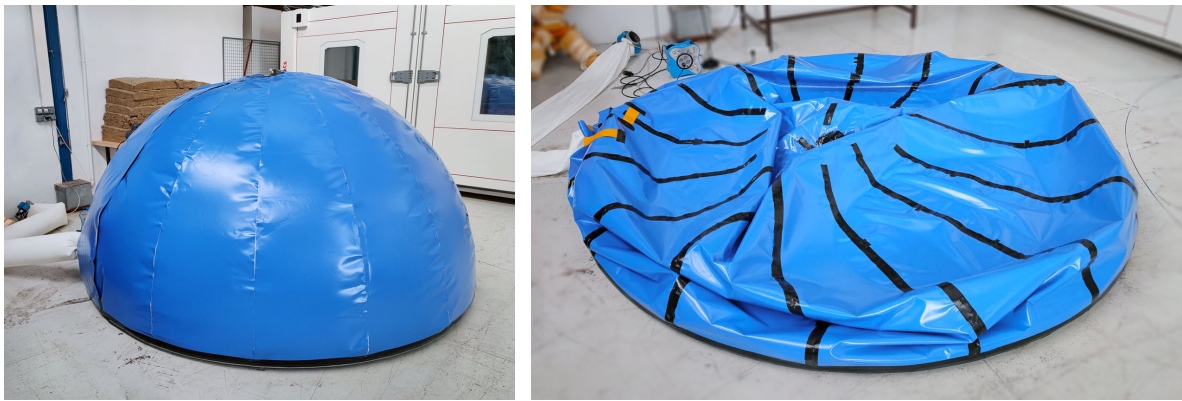
Figure 7.8: (left) Inflated dome with continuous air supply. The airtightness is not achieved yet, since only one layer of adhesive tape was applied inside. (right) Deflated dome with two layers of adhesive tape (on the inside and the outside).
