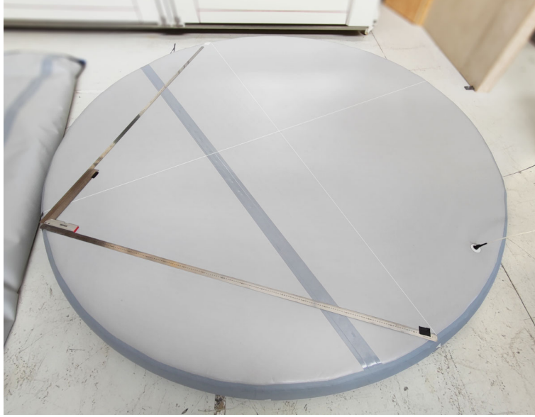
Figure 7.1: Geometric construction to mark two perpendicular diameters of a circular panel and mark its center.
