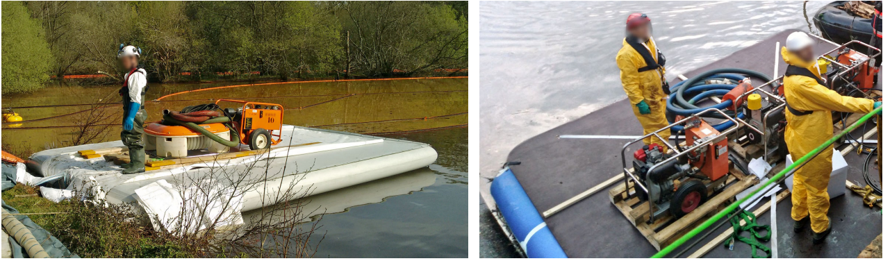
Figure 18: Floating decontamination platform, an example of real-world application of the buoyancy of inflatable panels. (© Écocréation)
