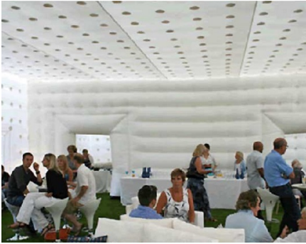
(a) Inflatable building with mattress walls.
