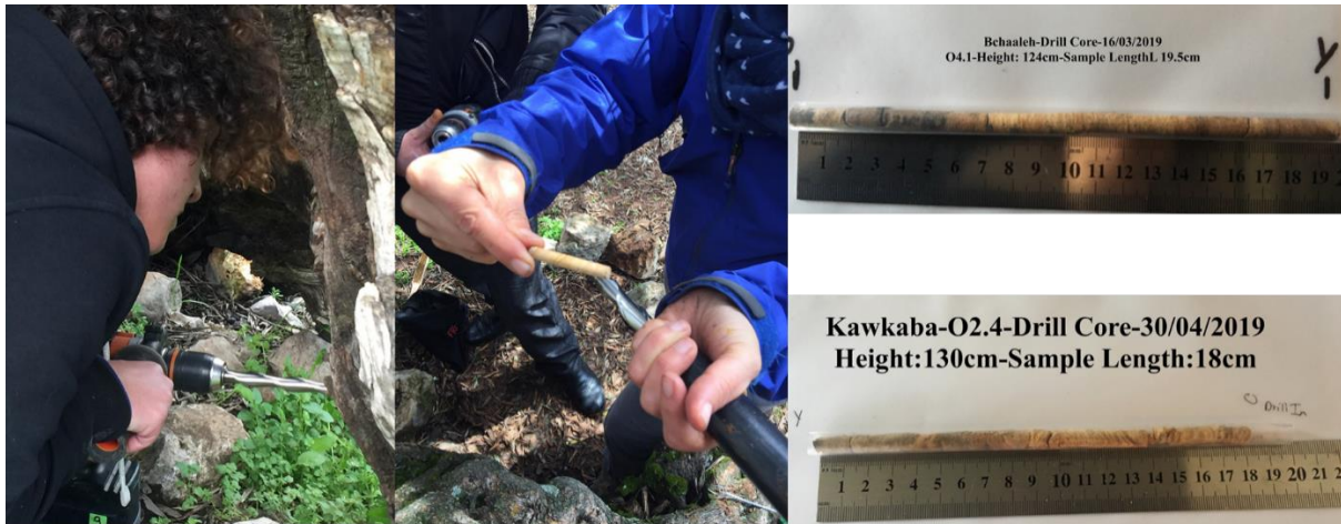
Figure 7 Wood core sampling using electrical driller.
