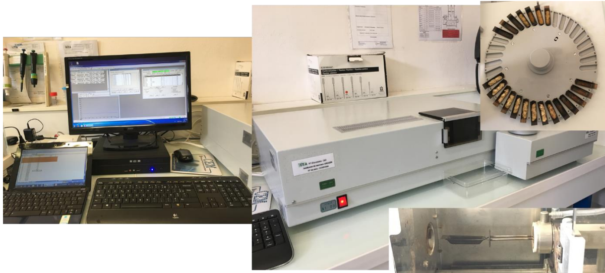
Figure 5 Advanced mercury analyzer AMA 254 at (IPREM).
