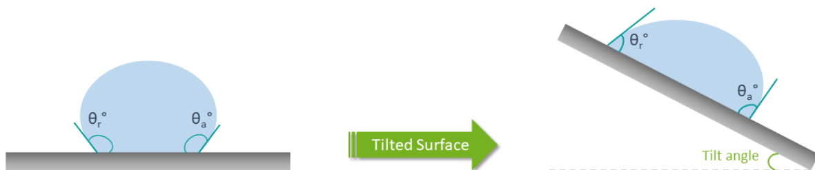
Figure 6. Receding and advancing contact angles determining contact angle hysteresis
