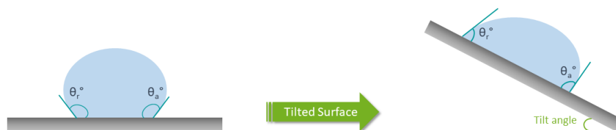
Figure 106. Diagram of the assessment of CAH by the tilting method.
