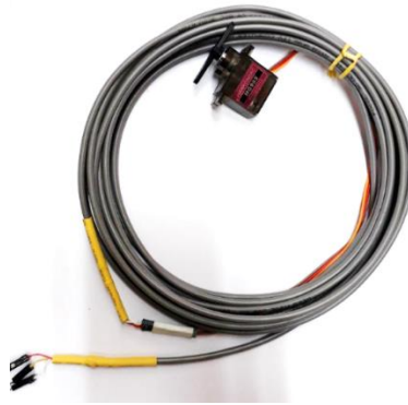
Figure 3.7. Micro-servomotor used for displacement of the laser.
