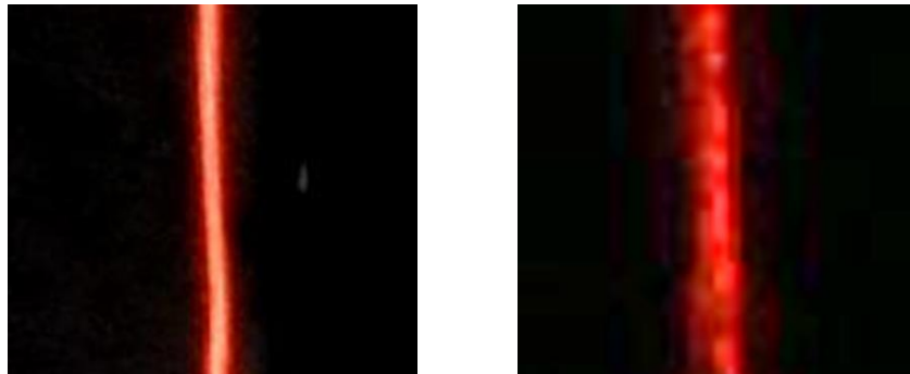
Figure 6.4. Light reflection around the light stripes taken by: Left) projector and Right) laser projection (the contrast has been ameliorated).
