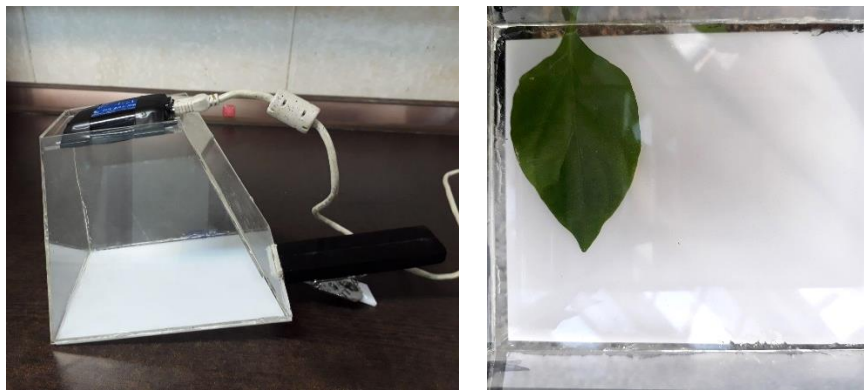
Figure 3.2. Hand-held leaf scanner and a sample image of a leaf.
