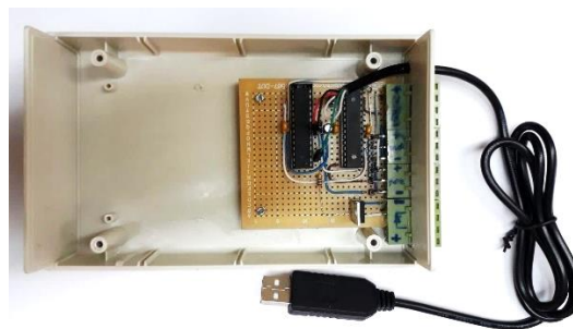
Figure 3.9. The controlling circuit of sensors.
