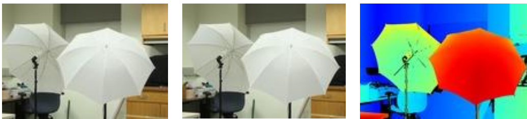
Figure 4.9. Sample left and right images with the disparity map.
