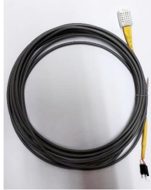
Figure 3.4. The temperature and moisture sensor.
