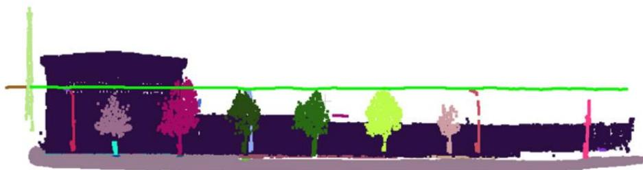
*Figure 2.13. An example of a segmented point cloud of a road surrounding (Xiang et al., 2018).*
