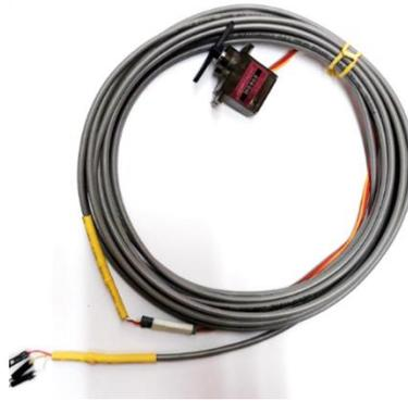
*Figure 3.7. Micro-servomotor used for displacement of the laser.*
