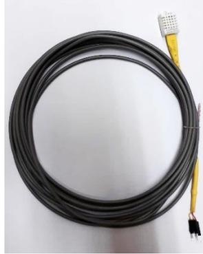
*Figure 3.4. The temperature and moisture sensor.*
