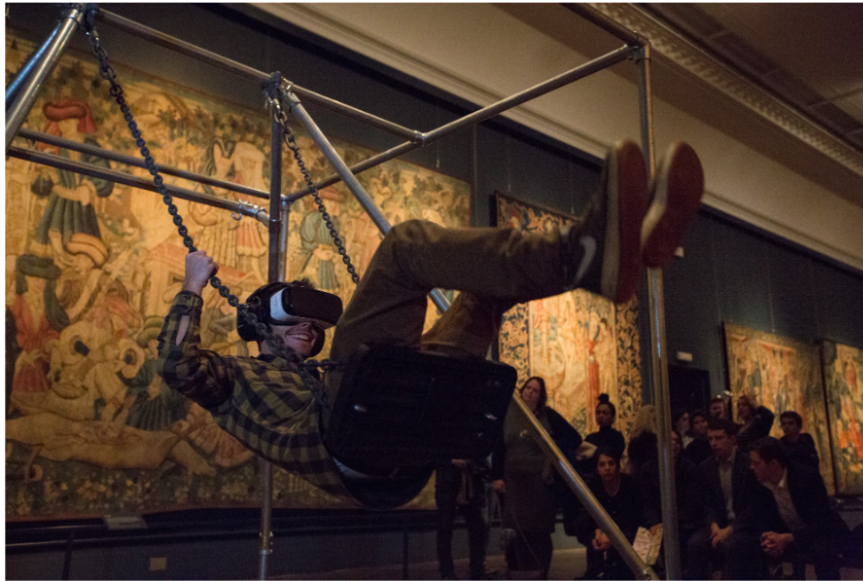
Figure 2.5: With Oscilatte [Tennent et al., 2017] the user has the illusion to realize faster swings and larger amplitudes. This visual-vestibular shift is detected but increases the sensations of the user.
