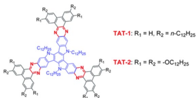
Figure 3.11 Molecular structure of TAT-1 and TAT-2. (Copyright from Qun Ye et al. [35])
