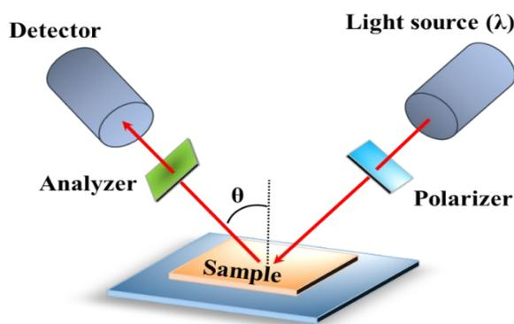
*Scheme A5.2 Schematic of spectroscopic ellipsometry.*
