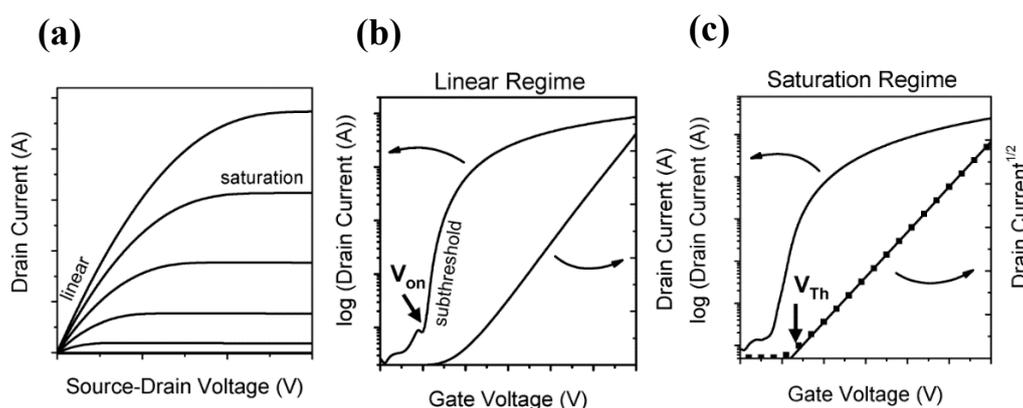
**Figure 6.3** (a) output characteristics indicating the linear and saturation regimes; (b) transfer characteristics in the linear regime, indicating the onset voltage ( $V_{on}$ ) when the drain current increases abruptly; (c) transfer characteristics in the saturation regime, indicating the threshold voltage  $V_{th}$ , where the linear fit to the square root of the drain current intersects with the x-axis. Reproduced from reference Zaumseil, J. et al, *Chem. Rev.* 2007, 107,1269-1323.
