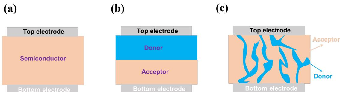
**Figure A7.2** Schematic of (a) single layer, (b) multilayer and (c) bulk heterojunction architecture OPV.
