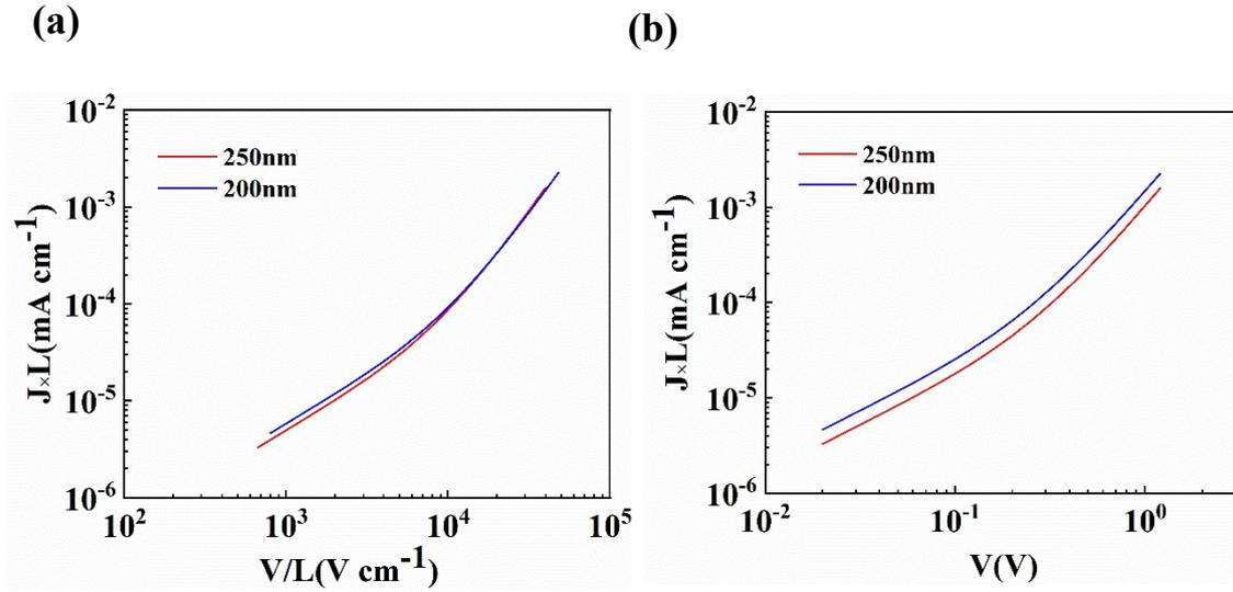
**Figure 6.5** *J-V characteristics of standard SCLC devices in the columnar-nematic state. (a)  $J \times L$  as function of  $V/L$ : the curves overlap in the SCLC part, as predicted by equation 1. (b)  $J \times L$  as a function of  $V$ : the curves do not overlap in the ohmic part, suggesting that the average background carrier concentration depends on the applied voltage.*
