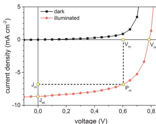
**Figure 2.13** Dark and illuminated  $J$ - $V$  characteristics of an organic solar cell. The point of maximum power ( $P_m$ ), as well as the two characteristic parameters, the short circuit current density  $J_{sc}$  and the open circuit voltage  $V_{oc}$  are marked in yellow. (Copyright from Tianyan Han.<sup>[85]</sup>)
