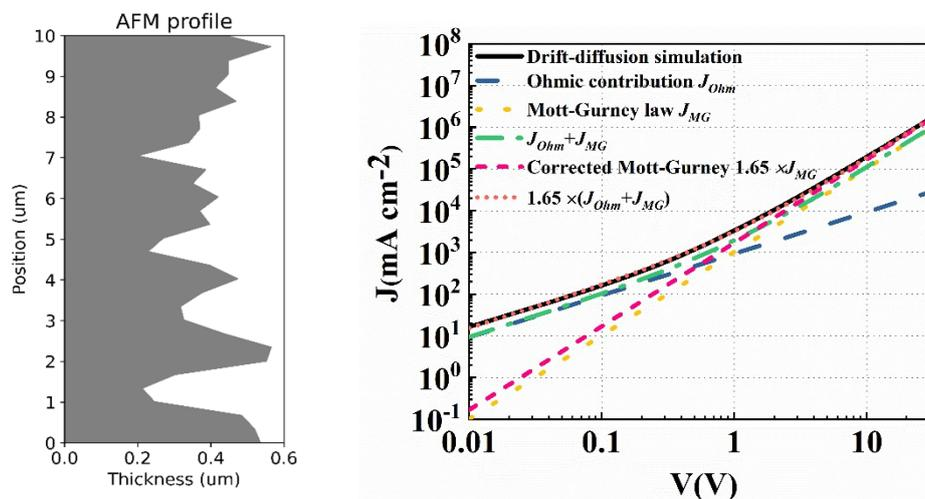
**Figure A6.2** Consequence of surface roughness on Mott-Gurney's law applicability. (a) AFM profile across a 10 μm wide representative region. (b) Simulated  $J$ - $V$  characteristics resulting from the rough profile.
