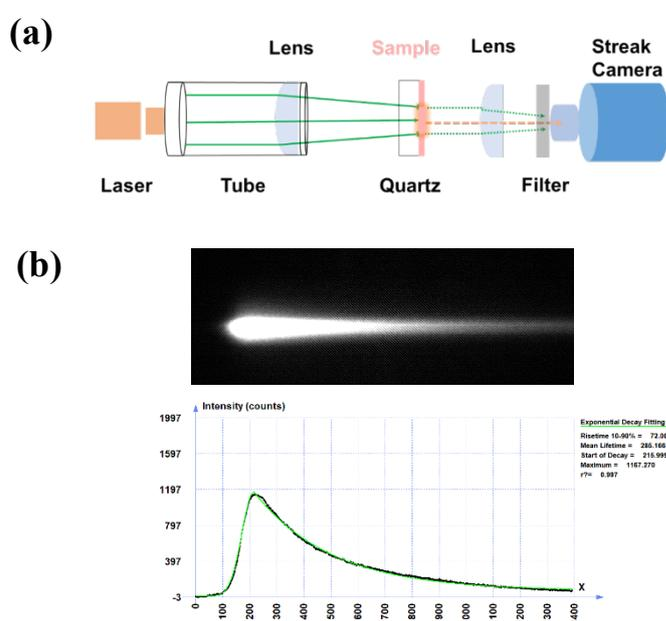
**Scheme 5.1** (a) Scheme of Time-resolved photoluminescence set up. (b) Top side: image registered through the slit of the streak camera as function of time (horizontally); Bottom side: graph of the PL intensity as a function of time extracted from the top image.
