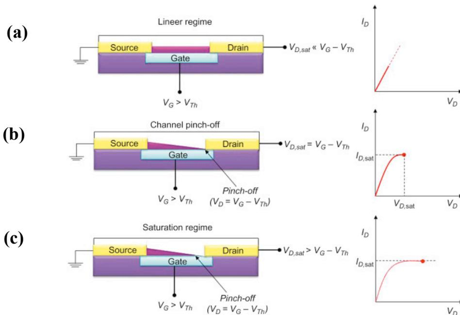
**Figure 6.2** OFET working conditions and corresponding current-voltage characteristics: (a) linear regime condition; (b) start of saturation regime at pinch-off; (c) saturation regime condition. (d) output characteristics indicating the linear and saturation regimes (copyright from Mahmut Kus, et al<sup>[28]</sup>).
