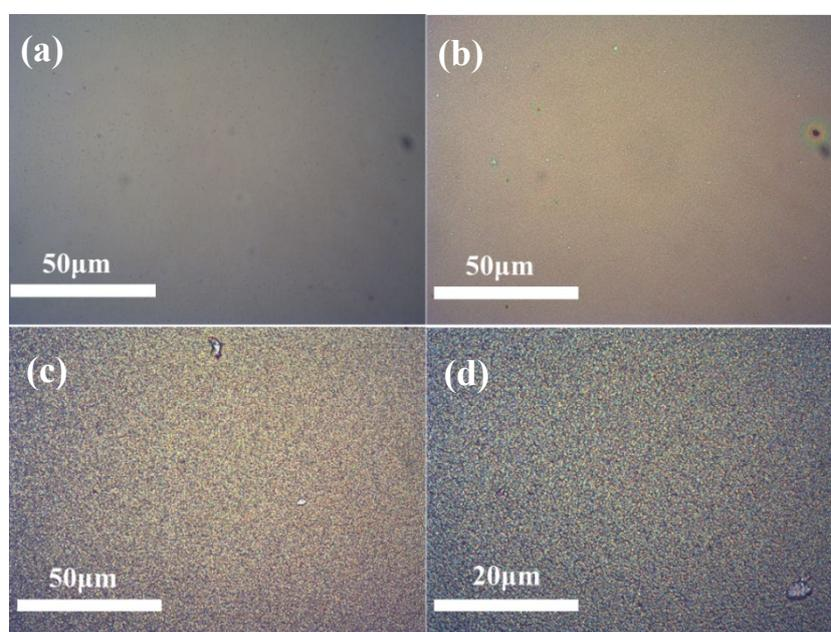
**Figure 7.5** Optical picture of BHJ solar cells based on  $TPD_{C8}-TAT_{C8}/P(NDI2OD-T2)$  under different annealing conditions: (a) as-deposited, (b) annealed at 145°C, 10 min, (c) annealed at 145°C, 40 min. (d) picture magnification 2.5 times (c).
