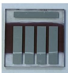
**Figure 7.2** Example of an organic solar cell device.
