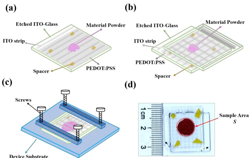
**Scheme A6.2** Thick SCLC devices. (a)-(c) Fabrication procedure of thick SCLC devices. (d) Image of thick SCLC device. For each sample, four efficient diodes were obtained with  $1.0 \text{ mm}^2$  individual active area (crossing of ITO stripes).
