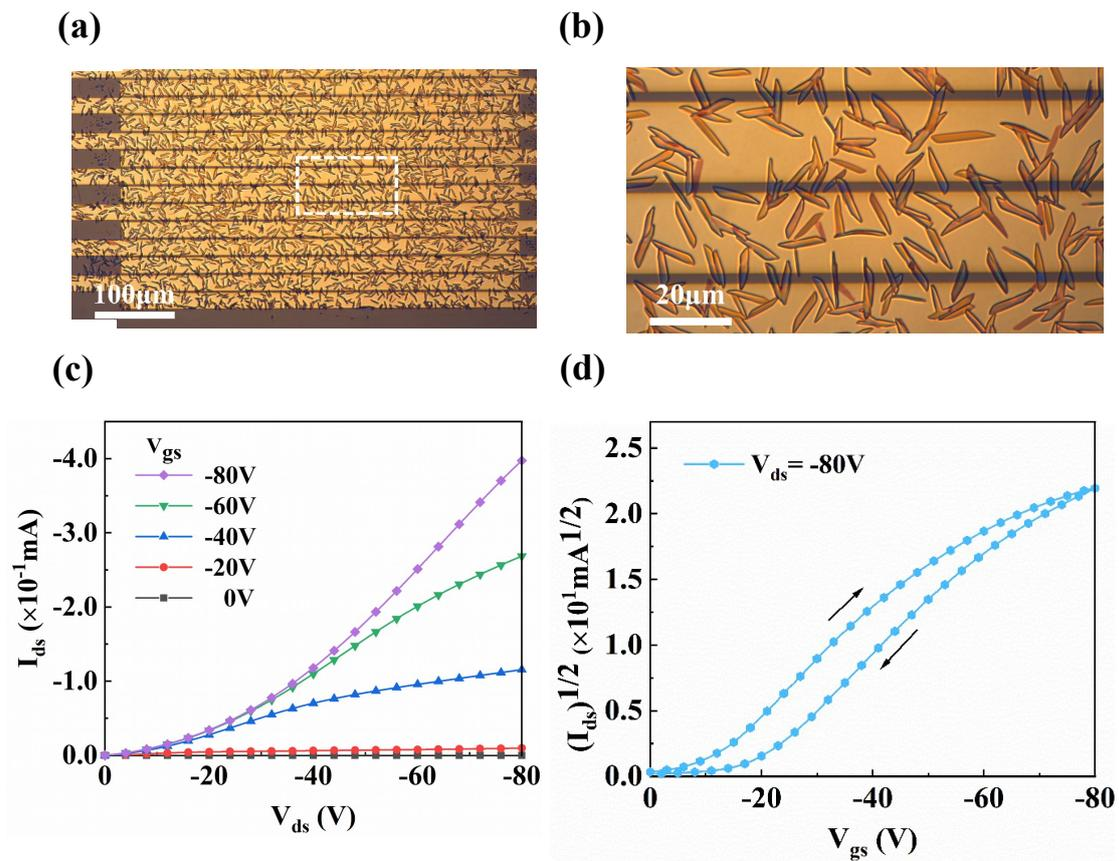
**Figure 6.10** (a) Optical micrograph of source and drain contacts of a bottom-contact-bottom gate transistor with TPDc8-TATc8 layer of large crystalline needles (channel length = 2.5 μm, channel width = 1.0 cm). (b) Zoom of dashed area in (a). (c) Output characteristics of the bottom-gate-bottom-contact OFET. (d) Transfer characteristics in the saturation regime.
