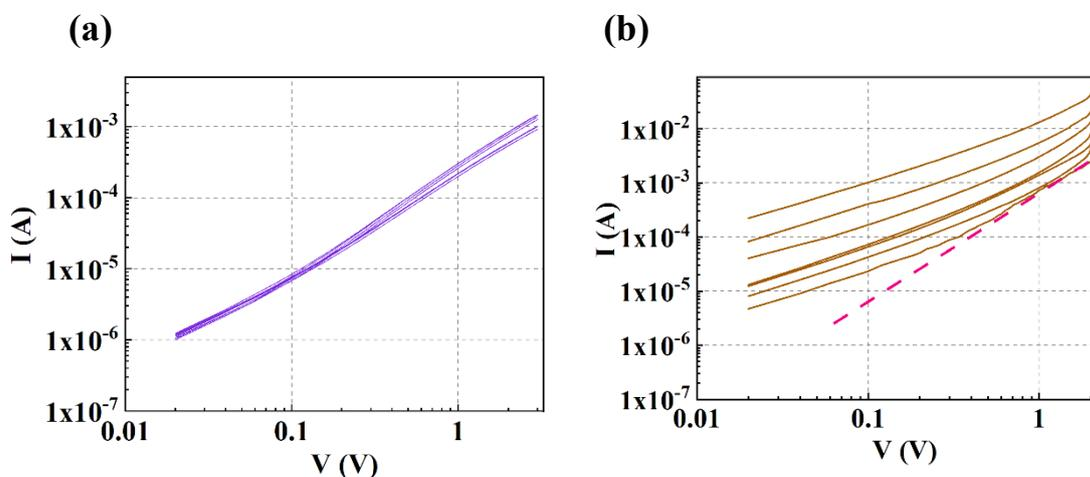
**Figure A7.3** I-V curve of (a) hole, (b) electron mobilities in the blends thin-films (condition c, Table 7.2).
