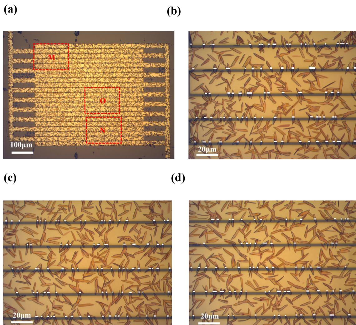
**Figure A6.4** Optical micrographs of bottom-contact-bottom-gate transistor with a 2.5 μm channel length and 1.0 cm channel width. (a) Full device. (b), (c) and (d) zoom  $\times 5$  of three regions used to estimate the fraction of channel width covered by the crystalline needles. The corresponding effective channel width is  $0.17 \pm 0.02$  cm.
