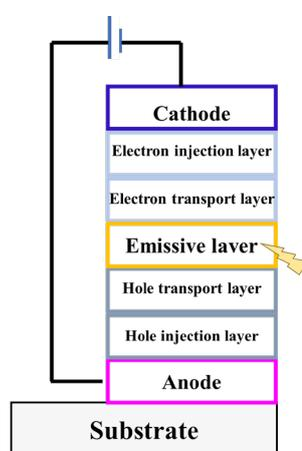
*Figure 2.10* Structure of an OLED device.
