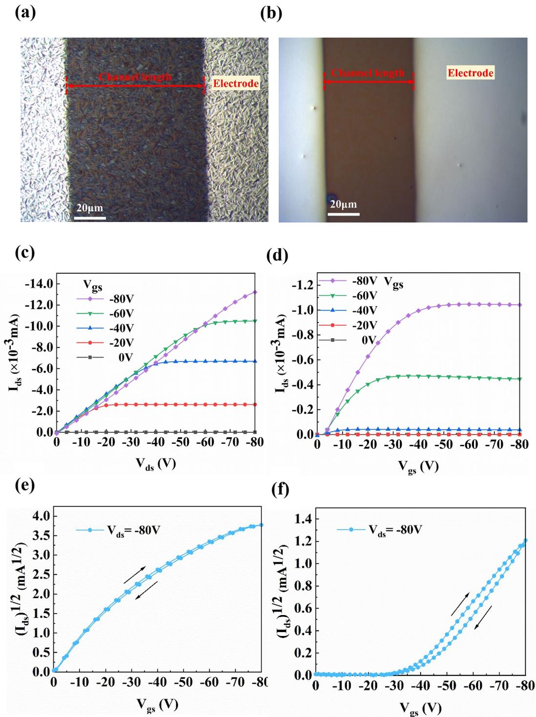
**Figure 6.9** Top-contact-bottom-gate transistor device. Optical micrographs of a transistor in (a) the crystalline state and (b) the columnar-nematic state. Output characteristics for (c) the crystalline state and (d) the columnar-nematic state. Transfer characteristics in the saturation regime for (e) the crystalline state and (f) the columnar-nematic state.
