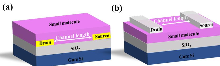
**Scheme A6.3** OFET device structures. (a) Bottom-contact-bottom-gate transistors, with ITO/Au bilayers used as drain and source electrode. (b) Top-contact-bottom-gate transistors, with  $\text{MoO}_3/\text{Ag}$  layers used as drain and source electrode.
