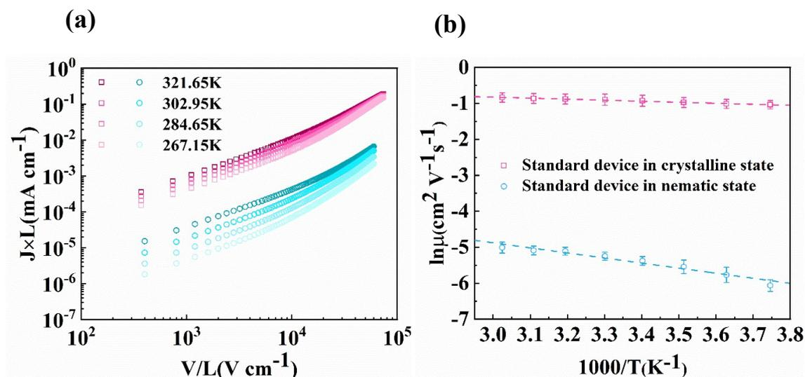
**Figure 6.8** (a)  $J$ - $V$  characteristics as a function of temperature on standard SCLC devices, in the crystalline state (open red squares) and columnar-nematic state (open blue dots). (b) Arrhenius plots of the hole mobility. Error bars are estimated from the measurements on four individual diodes.
