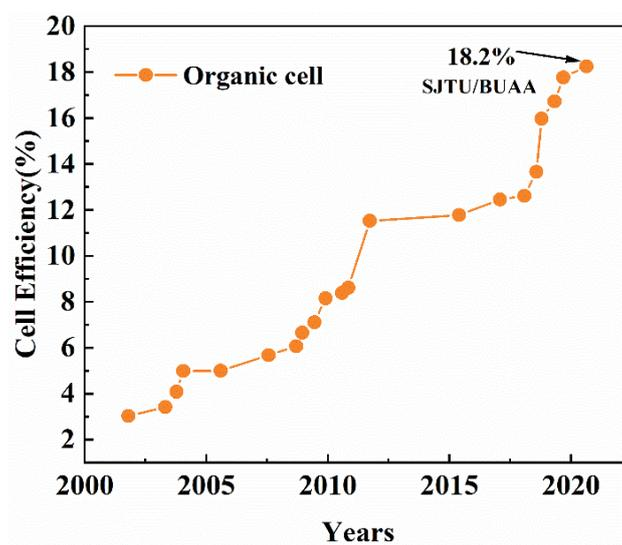
**Figure 2.14** Record efficiencies of organic solar cells based on organic molecular materials from 2000 to 2020. Data copyright: National Renewable Energy Laboratory Research Cell Efficiency Records (<https://www.nrel.gov/pv/cell-efficiency.html>).
