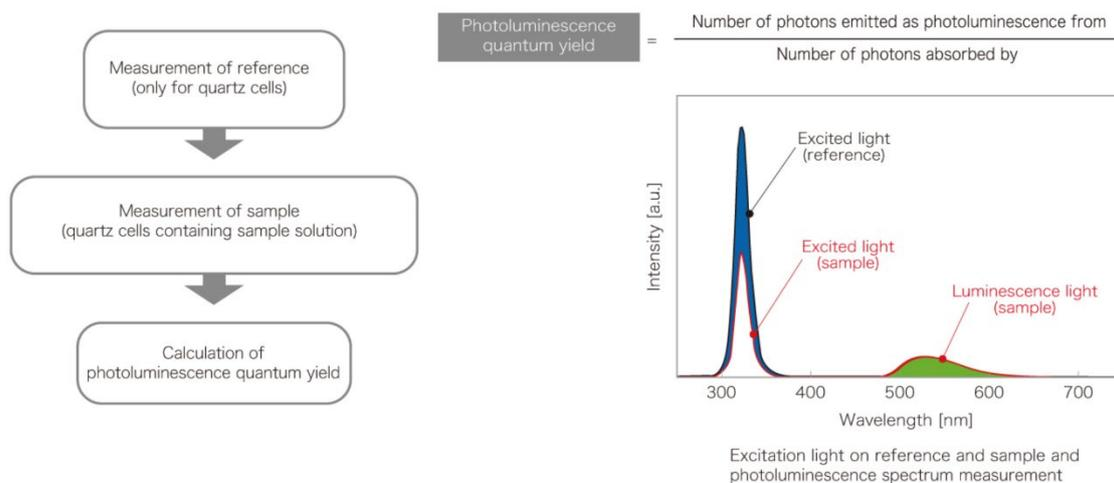
**Scheme A5.3** Principle of quantum yield measurement (copyright from <https://www.hamamatsu.com/eu/en/product/photometry-systems/luminescence-efficiency-measurement-system/quantaurus-xy/measurement-principle/index.html>).
