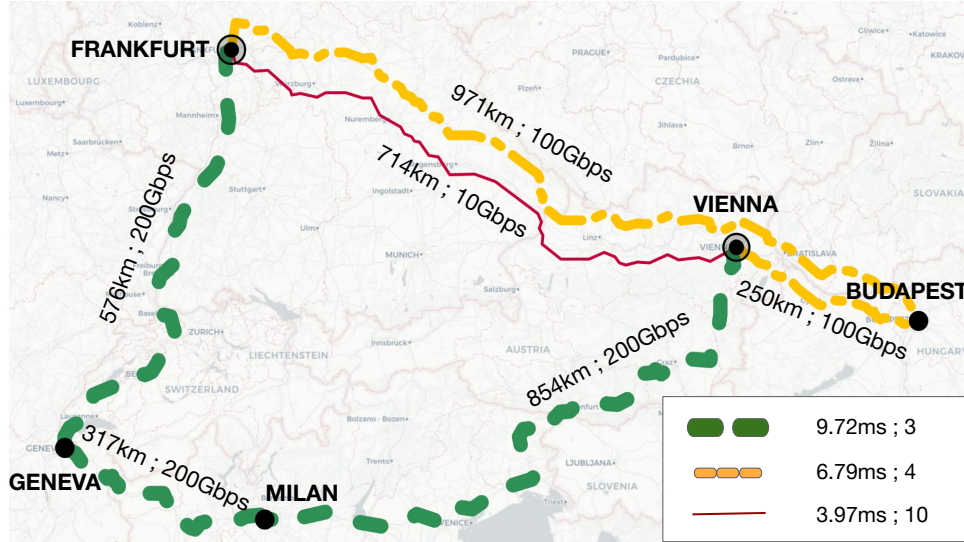
FIGURE 4.1: Practical relevance of DCLC in the GEANT network. IGP costs are deduced from the bandwidth of each link. Depending on their needs (in terms of delay and bandwidth), applications can opt for three non-comparable paths between Frankfurt and Vienna.
