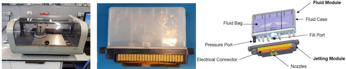
Figure 6. Screen-printer and cratridge used to print the membrane.
