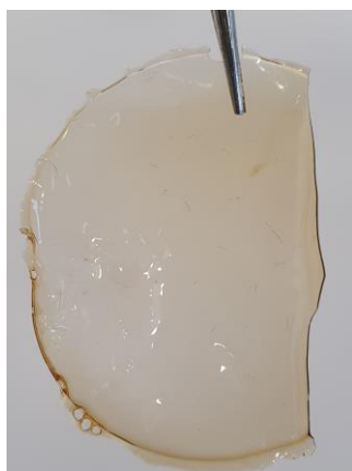
Figure 11. Membrane of fully sulfonated PPFS 0.77 -s-PMA 0.23 blended with 2 wt% of PBI.
