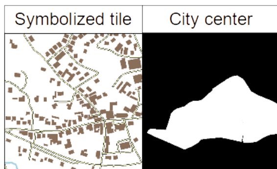
Figure C.23: Example of representation of the binary information location of city center with a black and white mask.
