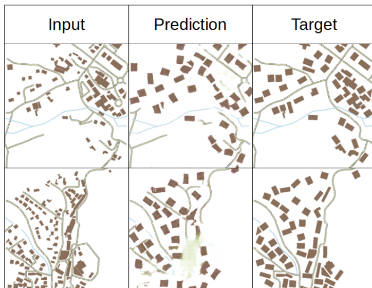
Figure F.10: Prediction of a model trained to generate a generalized map that includes road selection.
