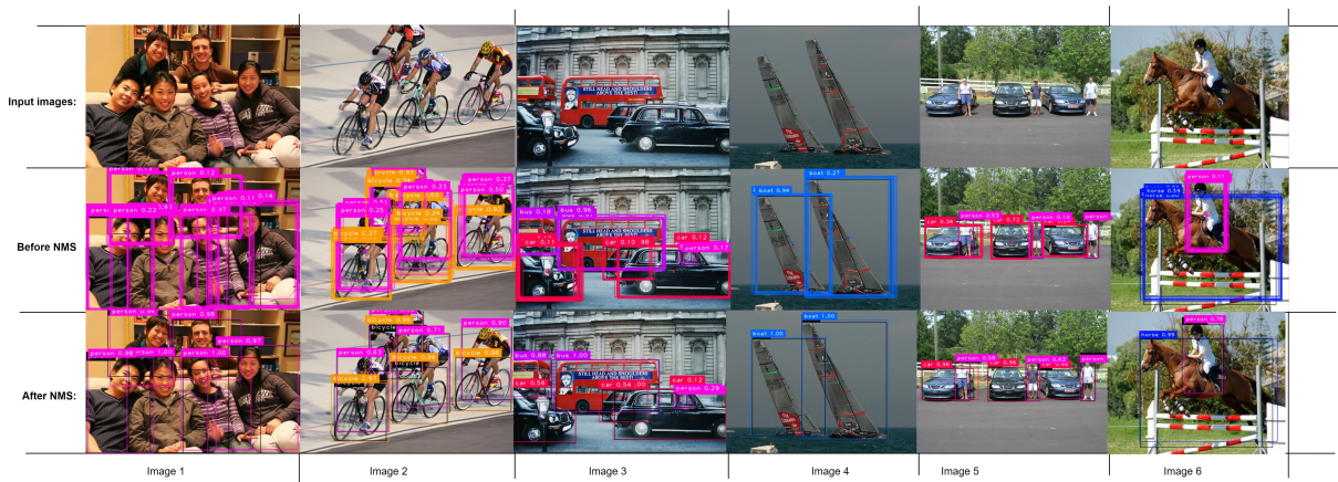
Figure 7.5: Sample MultiGridDet output on randomly selected Pascal VOC 2007 test set images. As seen from the figure the first row shows six input images, whereas the second row shows the prediction of the network before non-max-suppression (NMS) and the last row shows the final bounding box prediction of MultiGridDet on the input image after NMS thresholding.
