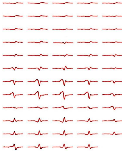
Figure 33: Example of a motor unit matched across knee flexion and ankle plantar flexion tasks. The figure depicts the distribution of the motor unit action potentials over the grid of electrodes during knee flexion (black curve) and ankle plantar flexion (red curve) for a gastrocnemius lateralis motor unit.
