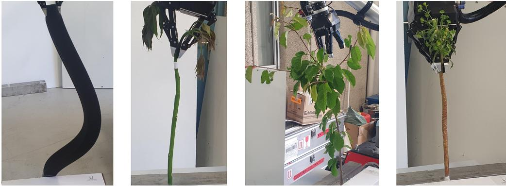
FIGURE 6.5: Different used objects in the performed experiments: a foam rod ( $L = 0.87$  (m)), three branches of different plants ( $L = 0.40, 0.60, 0.38$  (m))
