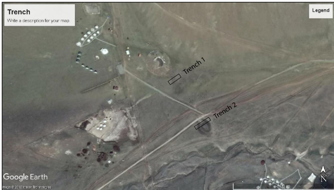
Figure 53. The locations of the two trenches in the Bumbat Valley of Mount Bogd Khan. The trenching locations were selected on the “open cracks” that might be tectonic related landforms. Trench 1: N47°50'1.62", 107°06'50.77"; Trench 2: N47°49'58.1", E107°06'53.3".
