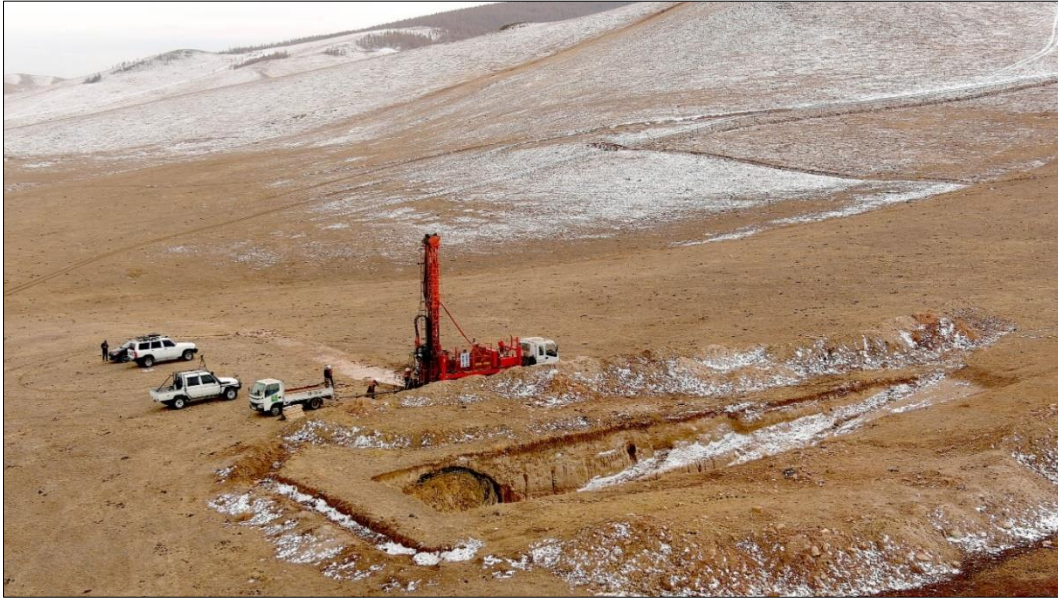
Figure 57. The vertical 90° drilling in ~5 m distance the eastern side of the east wall of the Khürel Togoot trench. November 3, 2021. Mount Bogd Khan, Ulaanbaatar.
