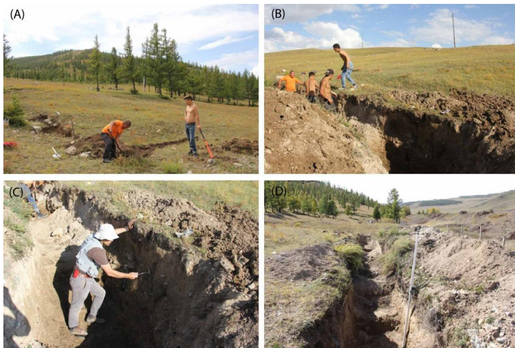
Figure 56. The trenches in the Tör Khurakh Valley of Mount Bogd Khan. The paleoseismological survey was conducted by the selecting 3 points on the satellite images that could be either the indistinct fault scarps or washout ravines (A, B, and D). (C)-the investigation process of the ditch walls.
