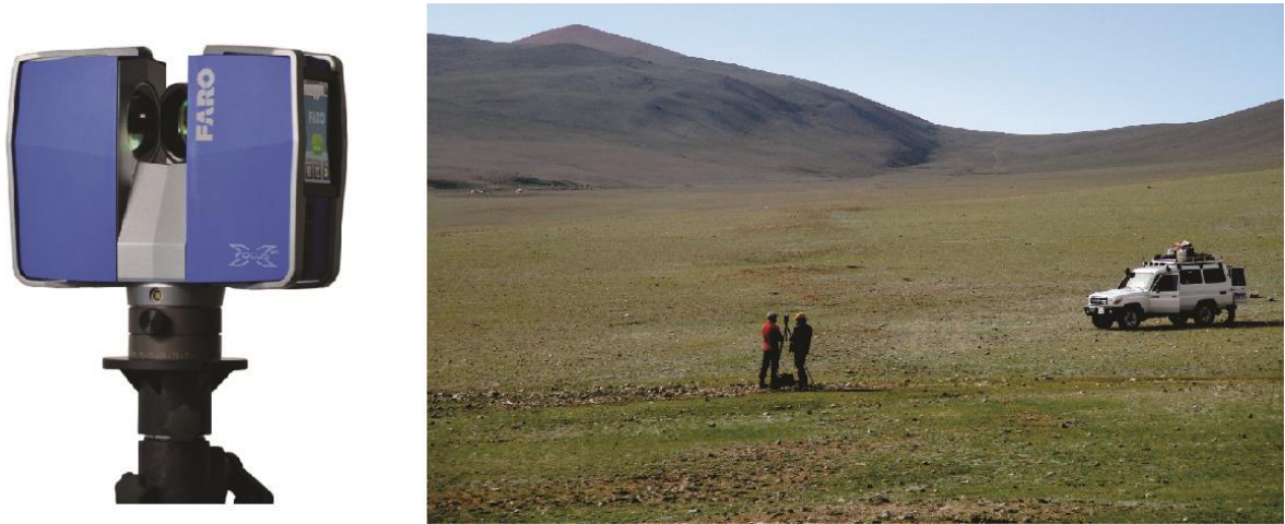
Figure 12. On the left, a photograph of “FARO Focus 3D X330” terrestrial laser scanner. On the right, a procedure of scanning a displaced gully in Davst Lake valley along the Ar-Khötöl surface rupture in July 2017.
