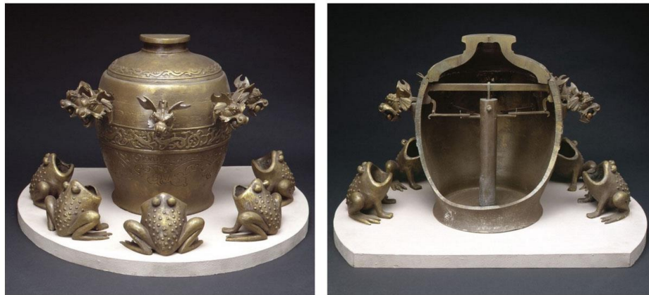
Figure 7. Chinese Astronomer Zhang Heng's seismoscope.
