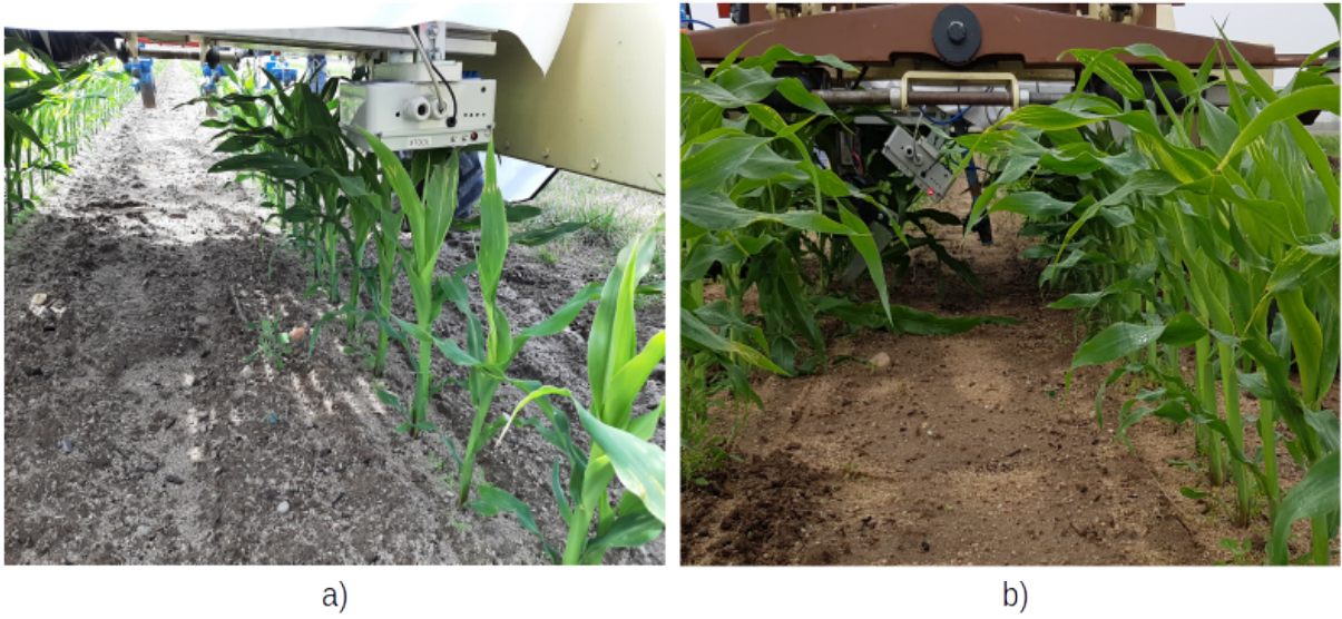
Figure 4.8: Xtool multimodal sensor. a) Obstruction of image acquisition. b) Xtool repositioning.
