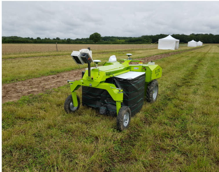
Figure 3.5: Multi-modal frontal detection onboard the experimental platform.
