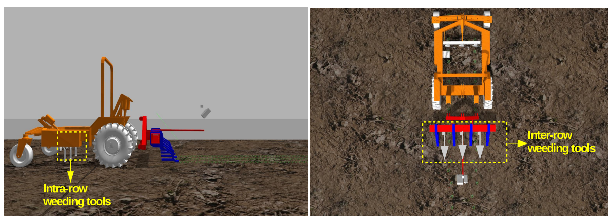
Figure 4.2: Mechanical tools placed in front and at the rear of the platform for inter-row and intra-row weeding.
