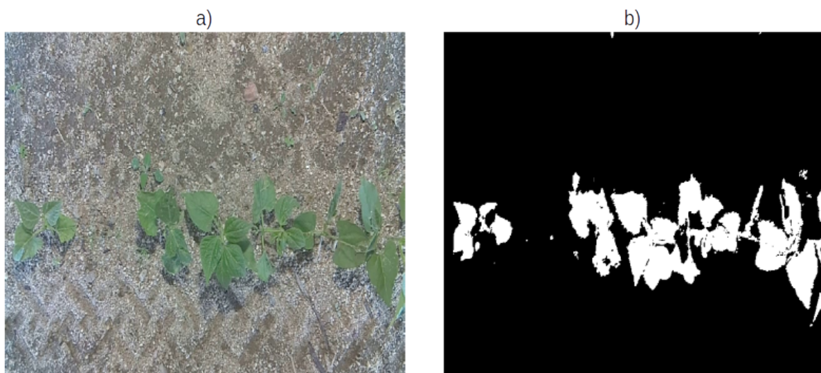
Figure 2.27: Bean mask generated by the algorithm based on physical characteristics. a) Original image. b) Bean mask.
