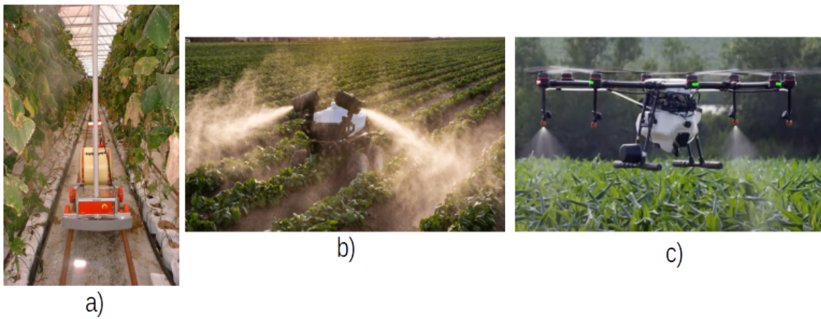
Figure 1.4: Examples of platforms to perform spraying task. a) Spraying robot designed by [15]. b) Spraying system R150-ATJ [16]. c) DJI octocopter AGRAS MG-1 [17].
