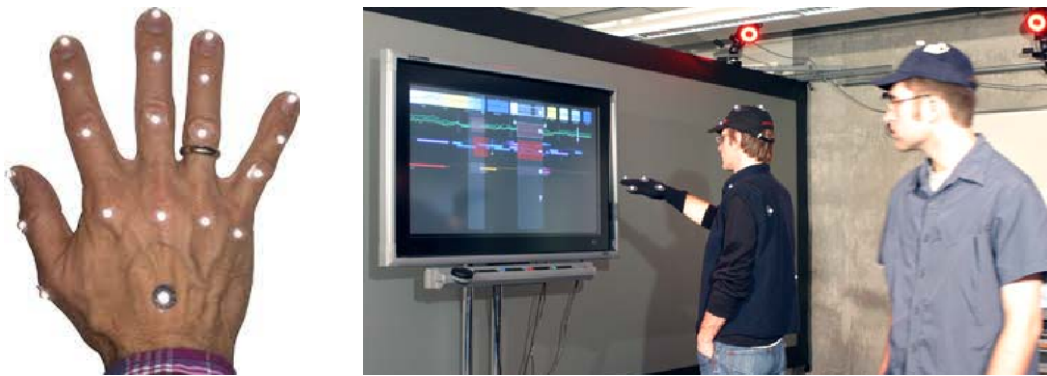
Figure 2.3: Examples of instrumentation for users to interact with mid-air bare hand gestures. On the left, 5mm infrared markers attached on the user hand to track precise gestures. On the right, users are equipped with a glove, a hat and a jacket with 10mm infrared markers attached to them to track their body, right hand, head and selected fingers. Images source: [147] and [215].
