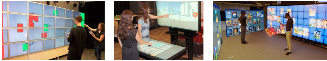
Figure 1.6: Large vertical screens used with other displays. On the left, tablets are used to control the cursors on the wall. In the middle, the user can position a tangible on a map displayed on a tabletop to display a street view of that location on a vertical display. On the right, users equipped with headsets to augment a wall display. Images source: [43], [51] and [108].
