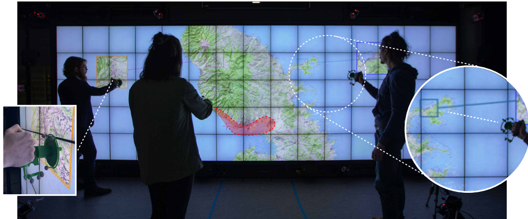
Figure 4.3: SurfAirs are custom physical controllers that users can manipulate both on the surface and in the air. In this scene, three users interact with SurfAirs : i) the user on the left uses a SurfAir as a surface controller, sliding and rotating it to pan and zoom in the inset window; ii) the user in the middle interacts from afar as she needs a wide view to perform a large lasso selection (in red); and iii) the user on the right is adjusting the position of the area to be magnified. He picked the viewport's proxy on the wall, and then stepped back to perform a large movement towards North-West without disturbing other users.
