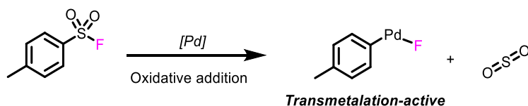
Figure III.1: Hypothesis of sulfonyl fluorides acting as base-free electrophiles in the Suzuki reaction
