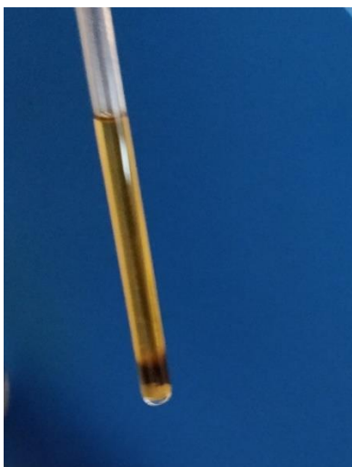
Figure 2.35: Formation of the three phases in the reaction mixture of 1.12 , lutidine and ytterbocene.
