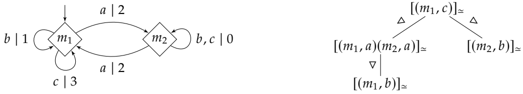
Figure 5.9: A parity automaton \mathcal{P} (left) with C = \{a, b, c\} and underlying structure \mathcal{M} used in Example 5.6.13. A diagram (right) showing the relations between the elements of \Phi_{\mathcal{M}}/\simeq ordered by partial preorder \triangleleft , discussed in Example 5.6.16.
