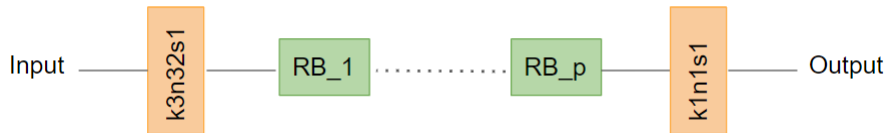
Figure 6.7: Architecture of the the first generator, where blocks RB_i, i = 1, \dots, p , are p residual blocks, k is the kernel size, n the number of filters and s the stride of the convolutional layers.
