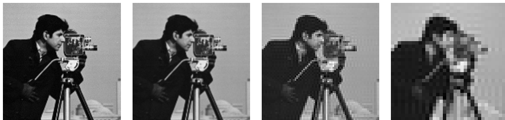
?figurename? 3.1: Cameraman image with different resolution from the left to the right: 272 \times 272 , 136 \times 136 , 68 \times 68 , and 34 \times 34 (keep noise and contrast level constant).
