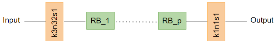
?figurename? 6.7: Architecture of the the first generator, where blocks RB_i, i = 1, \dots, p , are p residual blocks, k is the kernel size, n the number of filters and s the stride of the convolutional layers.
