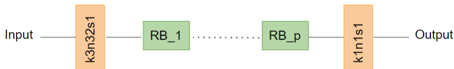
?figurename? 6.7: Architecture of the the first generator, where blocks RB_i, i = 1, \dots, p , are p residual blocks, k is the kernel size, n the number of filters and s the stride of the convolutional layers.
