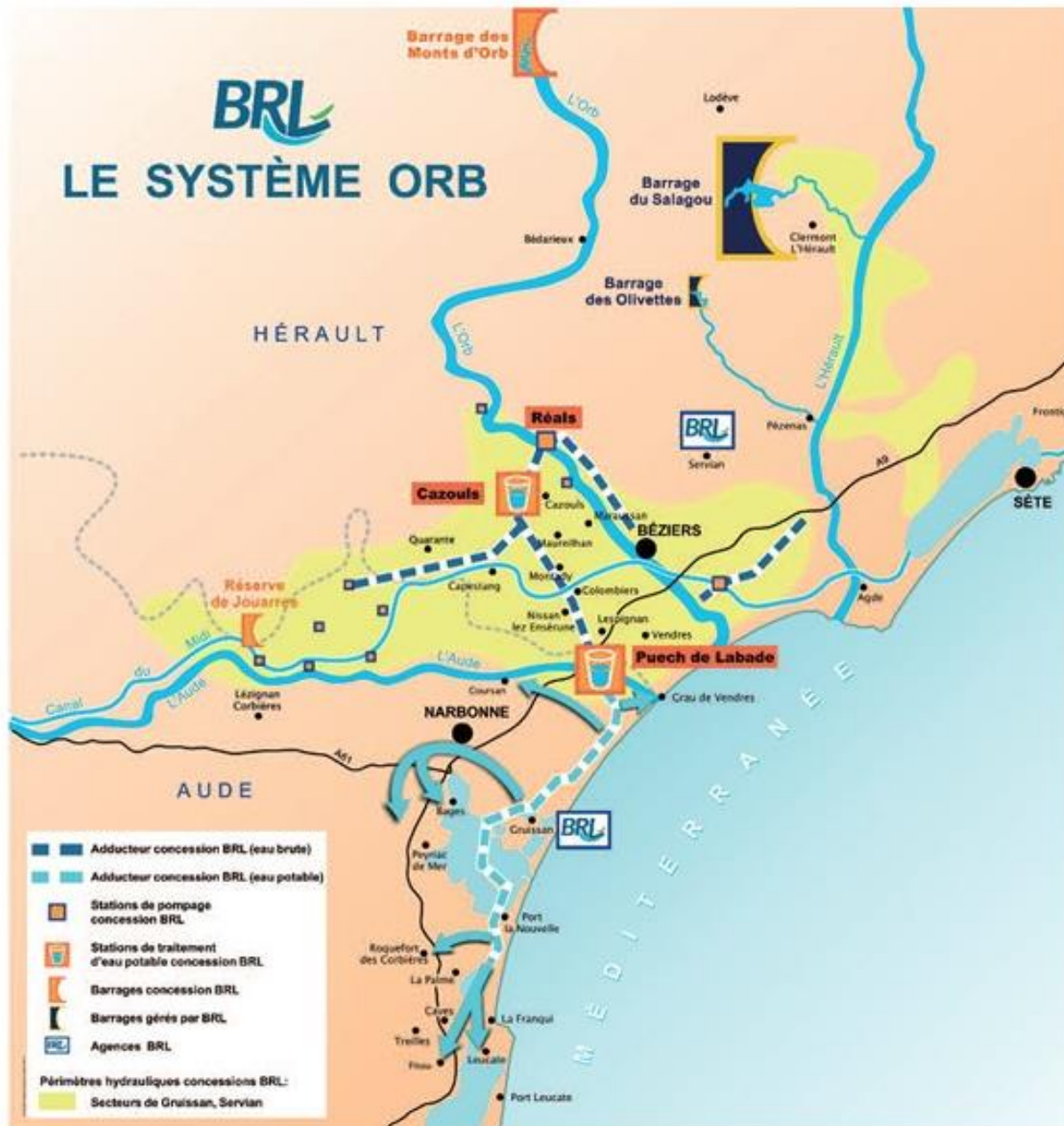
Figure 2.4. Orb water big infrastructures and main pumping stations (from BRL, 2009)
