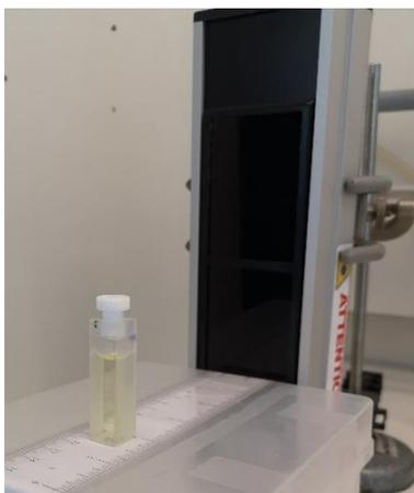
Figure 15 Irradiation setup with UV tubes for UV-Vis measurement.
