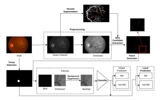
Figure 3.15: Pipeline for local prediction.
